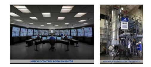
NuScale's safety design has been validated through rigorous testing of critical components, such as fuel assemblies, control rod and control rod mechanisms and the integral helical coil steam generators. NuScale has constructed an electrically-heated, one-third scale, full-pressurized and temperature integral thermal-hydraulic test facility that demonstrates the operation of the entire nuclear steam supply system and safety systems.
